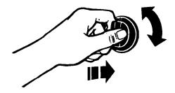
Until you get used to the settings, use the following as a guide. For best results, start cooking at the high setting; then turn the control knob down to continue cooking.
